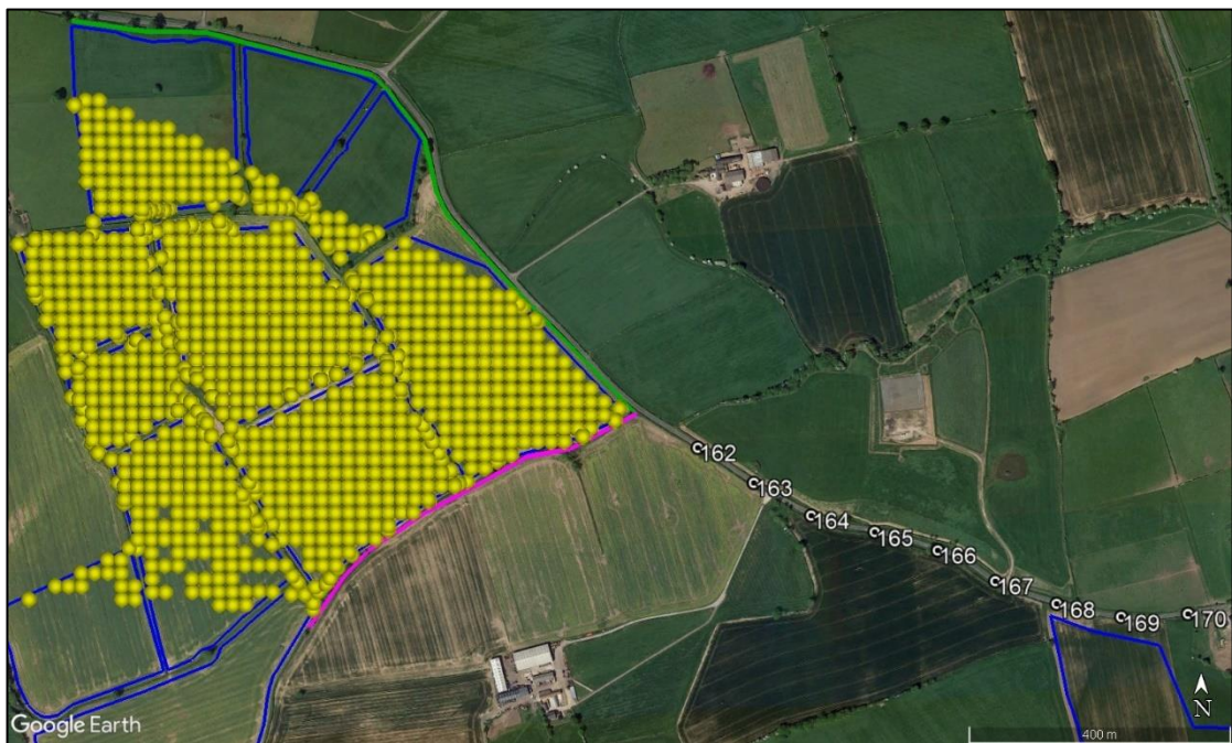
Figure 65 Critical proposed hedgerow/tree planting (pink line) relative to reflectors (yellow icons) for road section 162-170
