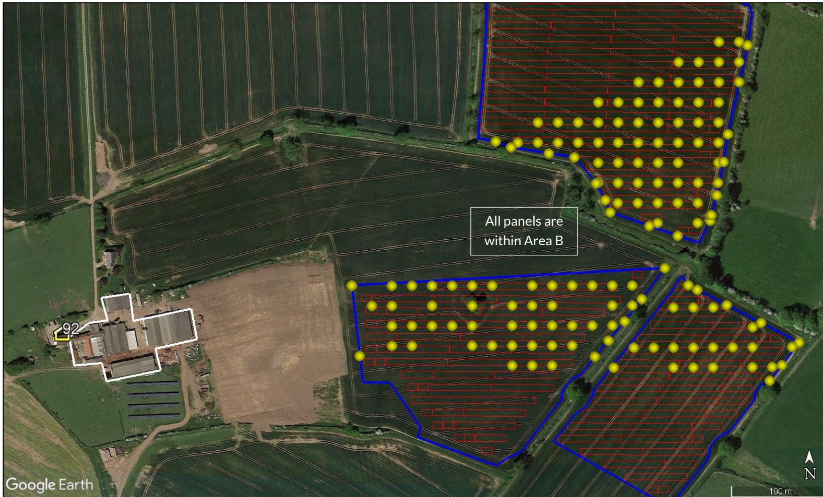
Reflecting points (yellow icons) and significant building/vegetation screening (white polygon) for dwelling 92
