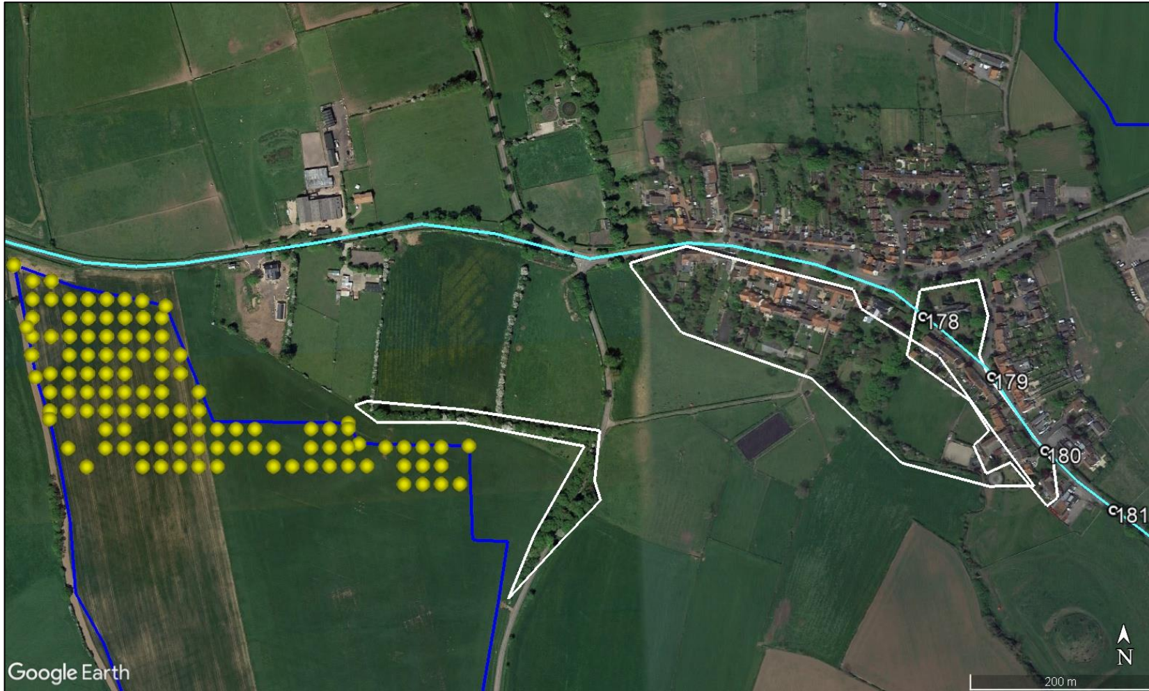
Reflecting points (yellow icons) and significant building/vegetation screening for road section 178-181
