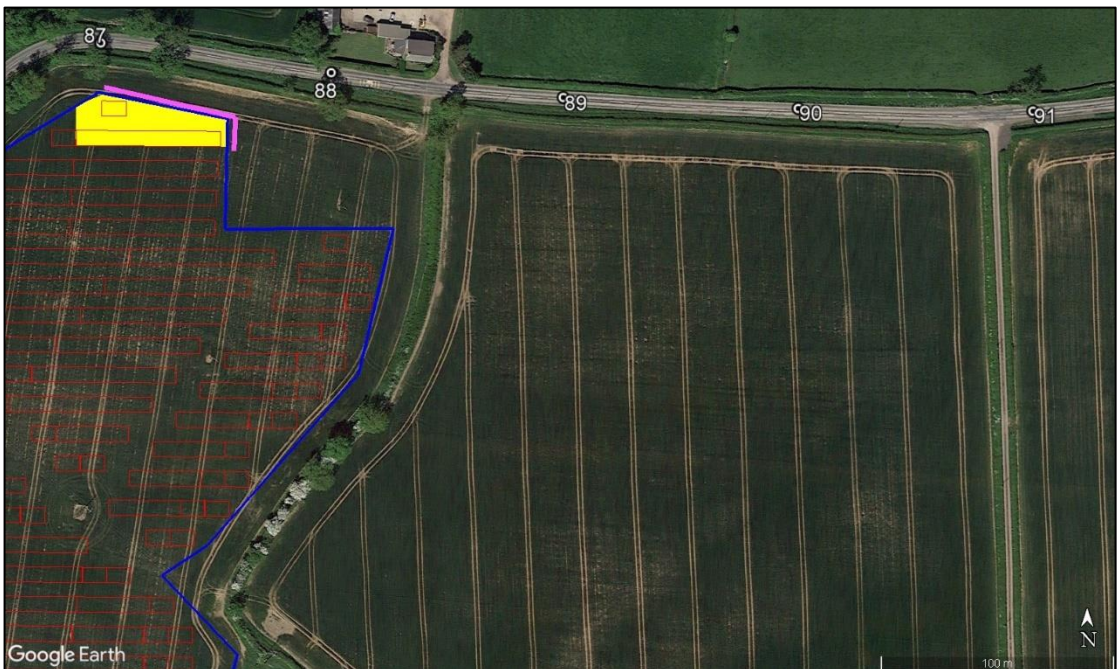
Figure 63 Critical proposed hedgerow/tree planting (pink line) relative to reflecting area for road section 90-91 (pink line)
