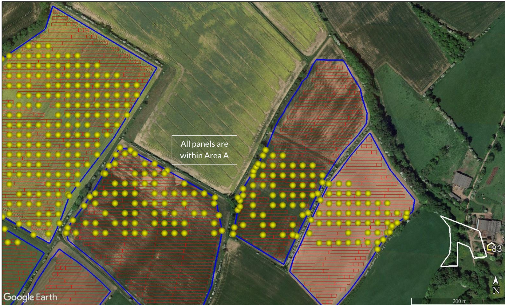
Reflecting points (yellow icons) and significant building/vegetation screening (white polygons) for dwelling 83
