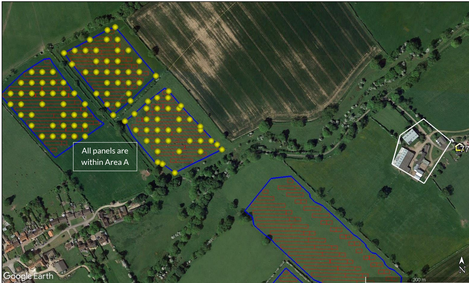
Reflecting points (yellow icons) and significant building/vegetation screening (white polygon) for dwelling 77
