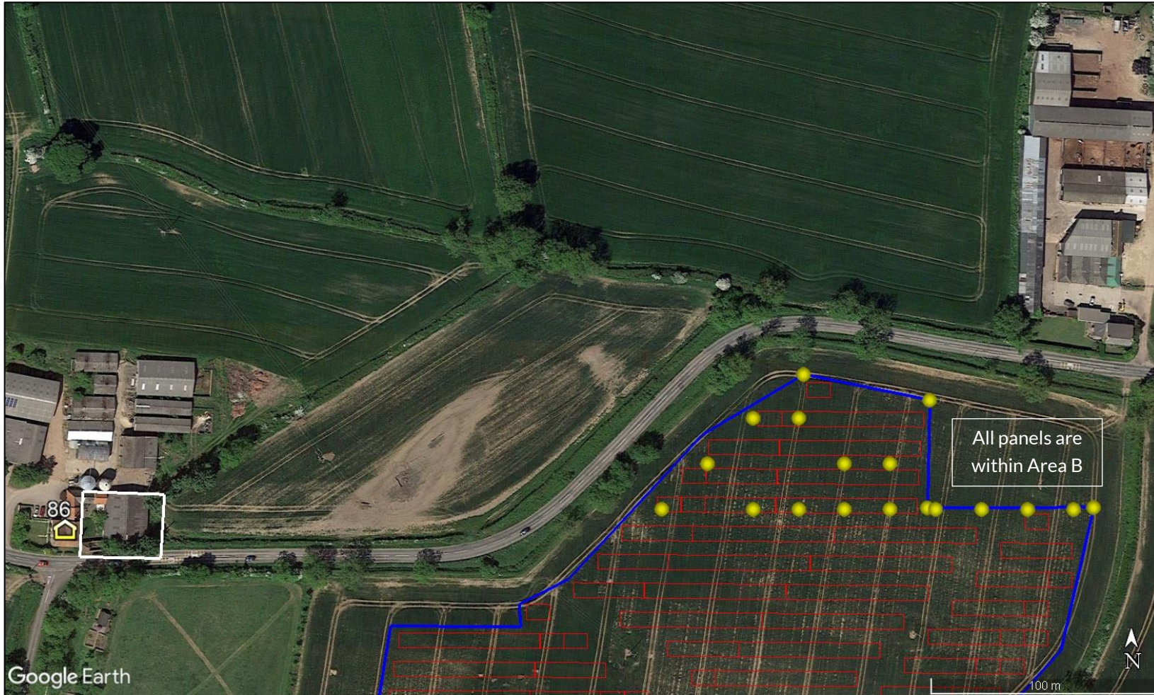
Reflecting points (yellow icons) and significant building/vegetation screening (white polygon) for dwelling 86
