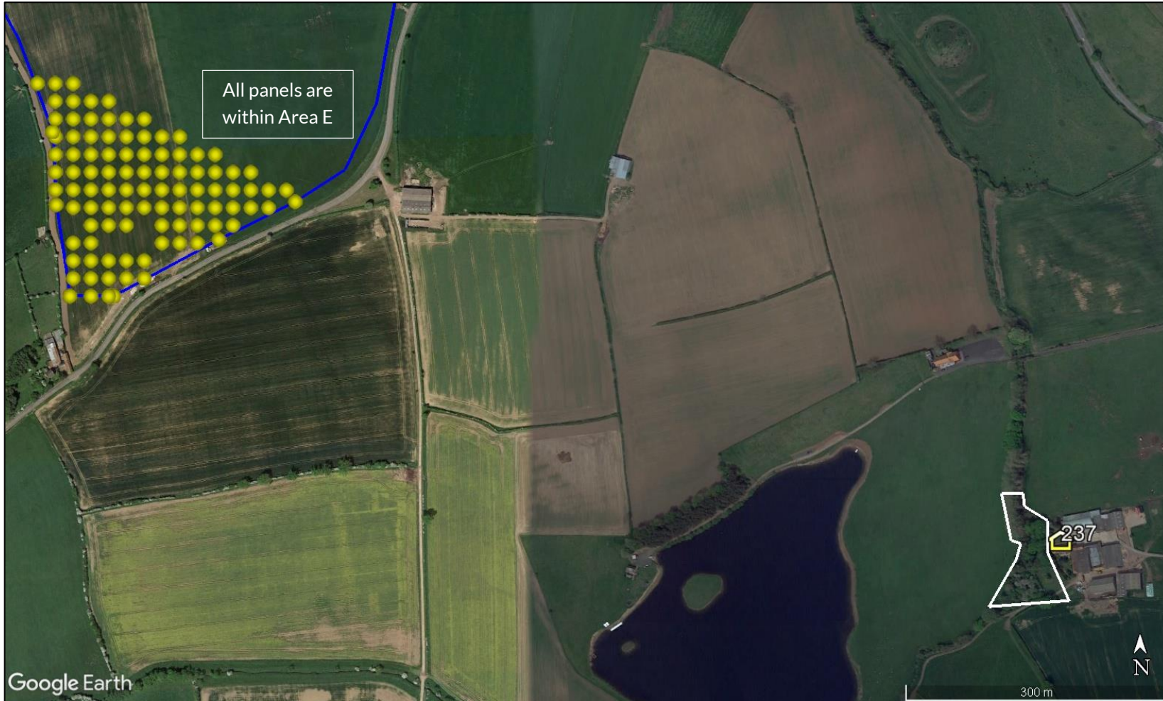
Reflecting points (yellow icons) and significant vegetation screening (white polygon) for dwelling 237
