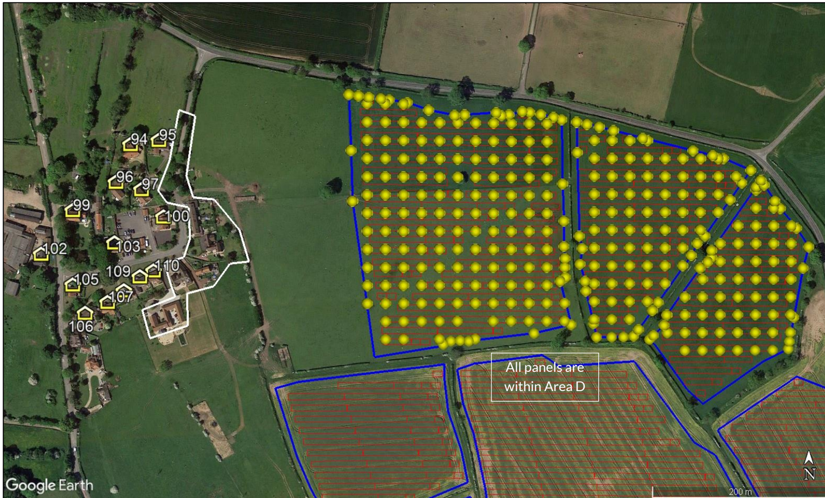
Reflecting points to the east (yellow icons) and significant building/vegetation screening (white polygon) for dwellings 94-97, 99-100, 102-103, 105-110
