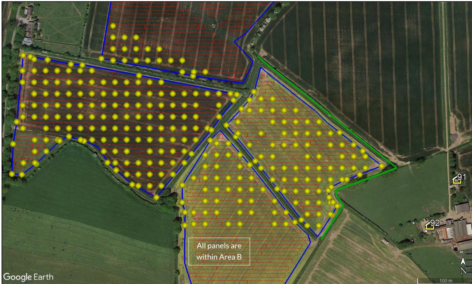
Reflecting points (yellow icons) for dwellings 91 and 92 and proposed hedgerow/tree planting (green lines) expected to provide screening
