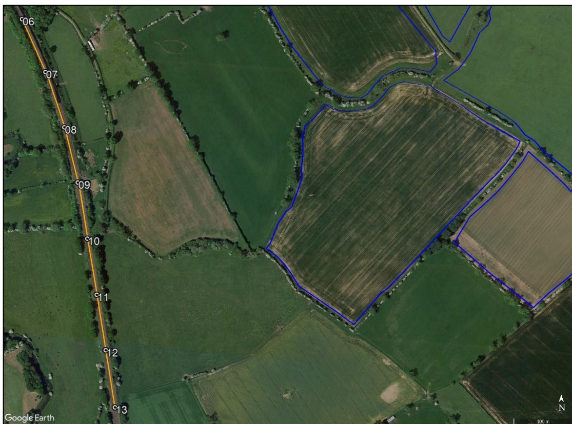
Figure 61 Section of railway towards which solar reflections are geometrically possible (orange) – aerial image
